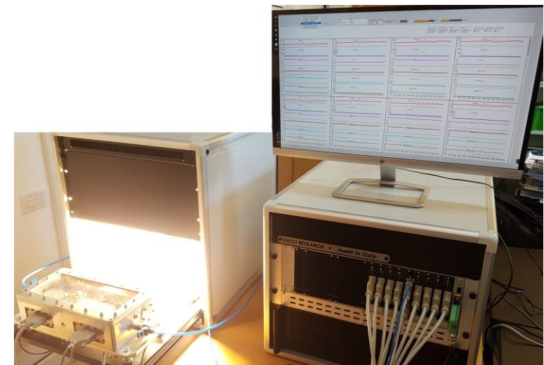
Multichannel platform with programmable light soaker and environmental chambers
